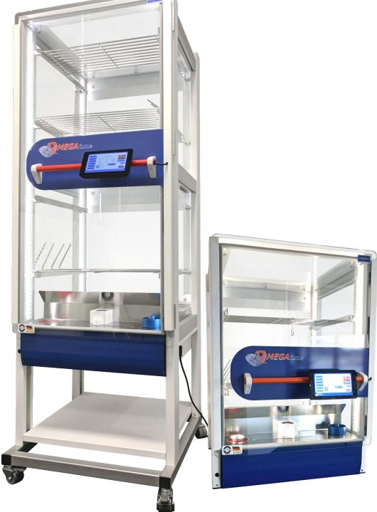
fingerprint fuming chamber series for cyanoacrylate development of fingerprints on non-porous surfaces
